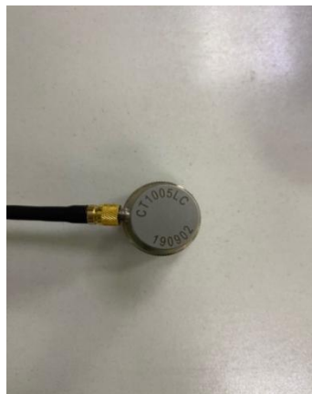
Fig 4: CT1005LC acceleration sensor
