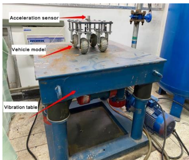
Fig 5: Shaking table test diagram
